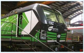
In the second half of 2016, our workshop in Ljubljana took up maintenance of the Vectron electric locomotives owned by European Locomotive Leasing (ELL). Our team are certified by the Austrian maintenance supplier ÖBB – TS to supply N30 control checks, also known as P1 checks, which are carried out after every 30,000 km in service.
