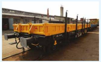
In 2016, we once again received an order by our Czech customer LOKO TRANS for an overhaul of 12 Regmms freight wagons. The work included a G4.0 overhaul, complete painting of all 12 units, replacing the timber floor with metal panels, installing wagon sidewalls, and adding a new exterior design for the end customer.
