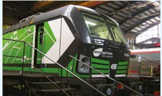
In the second half of 2016, our workshop in Ljubljana took up maintenance of the Vectron electric locomotives owned by European Locomotive Leasing (ELL). Our team are certified by the Austrian maintenance supplier ÖBB – TS to supply N30 control checks, also known as P1 checks, which are carried out after every 30,000 km in service.
