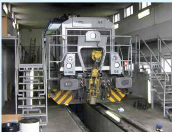
monitoring electronics system. Although the second inspection required significantly more work than the initial one, and the maintenance of the locomotive being a first-time experience, our team completed the task without any difficulties. Since then our Divača team is providing Port of Koper with regular maintenance services of the locomotive.
