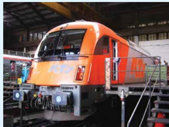
One of their locomotives, a Siemens Taurus (ES 64 U4) electric locomotive labelled Class 1216-901, arrived to Center Ljubljana for a P12 control check all the way from Croatia, where it runs service on a track-renewal construction site. As this particular model is almost identical to SŽ Class 541, the work on the orange newcomer largely followed the usual practice applied to SŽ locomotives of this type.
