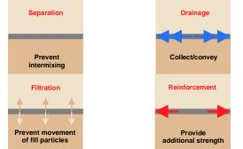
Figure 1: Principal Geosynthetic functions in rail
