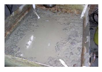
Figure 11: Excavated/failed formation in 'derby' rig
