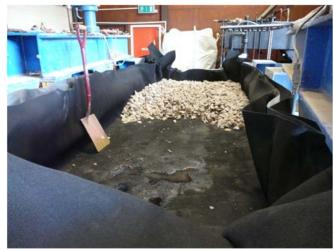
Figure 14: Installing prototype composite and ballast
