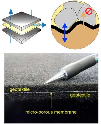
Figure 17: Geocomposite filter
