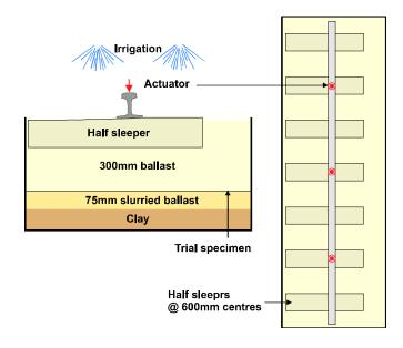
Figure 12: Test set-up on large rig
