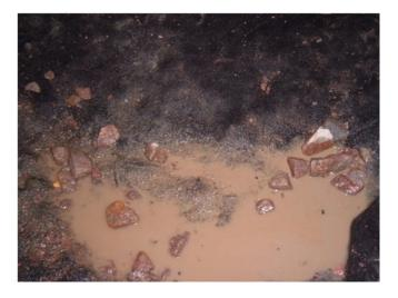
Figure 15: The upper side of the composite after 70MGT loading
