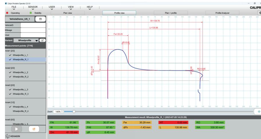
Example display of the measured variables in the CALIPRI Portable Operator (CPO)
