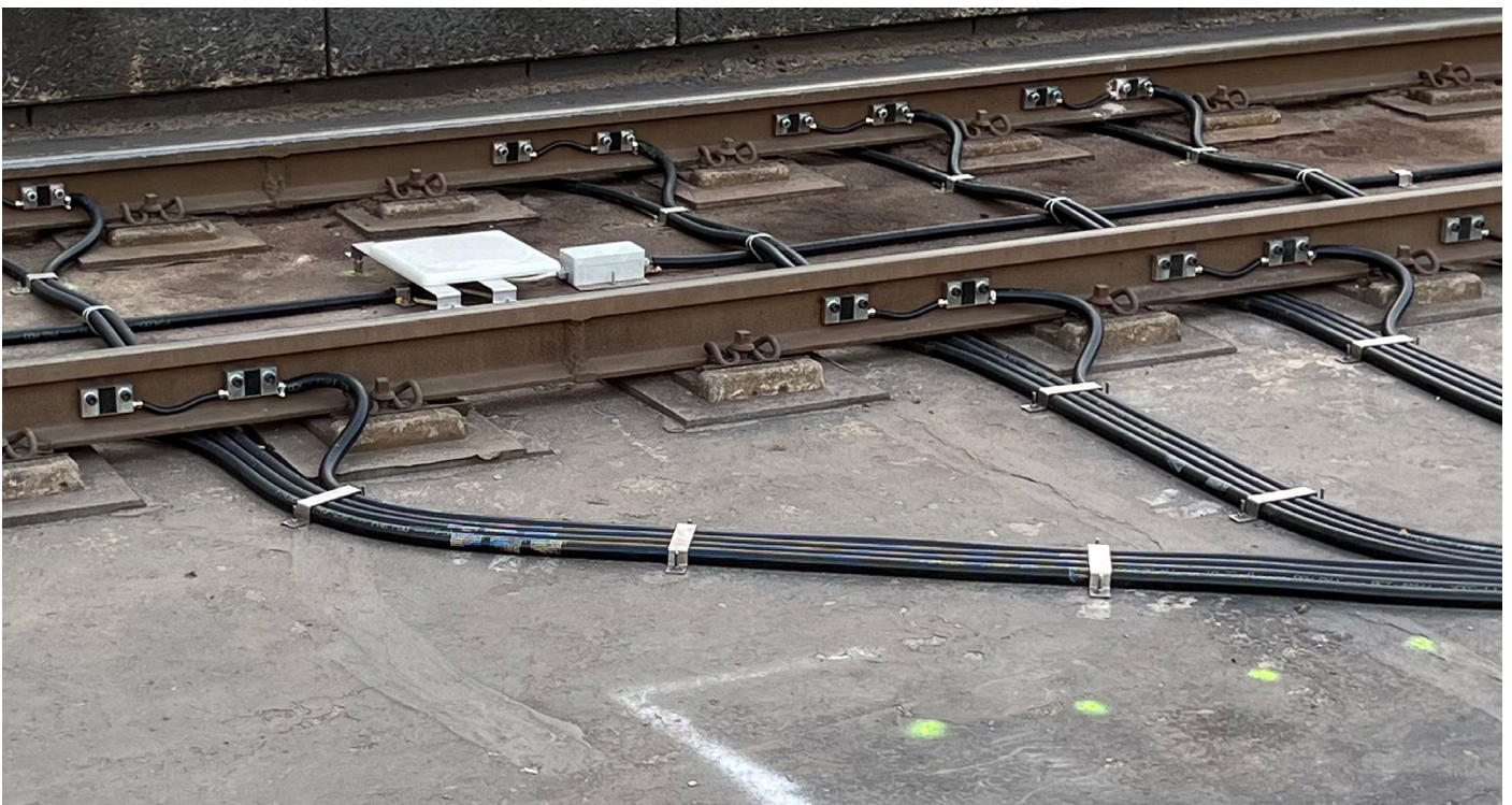
Dynamic Weighing System: measures axle loads, wheel loads, total tram weight and balance dynamically as trams pass at regular speeds
