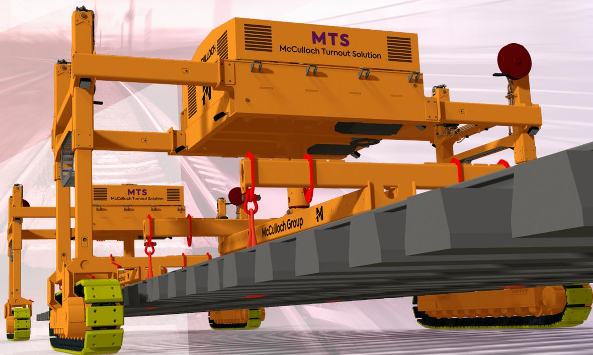
**The MTS can access and egress almost anywhere on track.** It can move with ease pre-built panels in any direction before installation, allowing you to handle S&C installation with ease. The MTS also removes the need for large work areas, or temporary track along with associated planning challenges.
