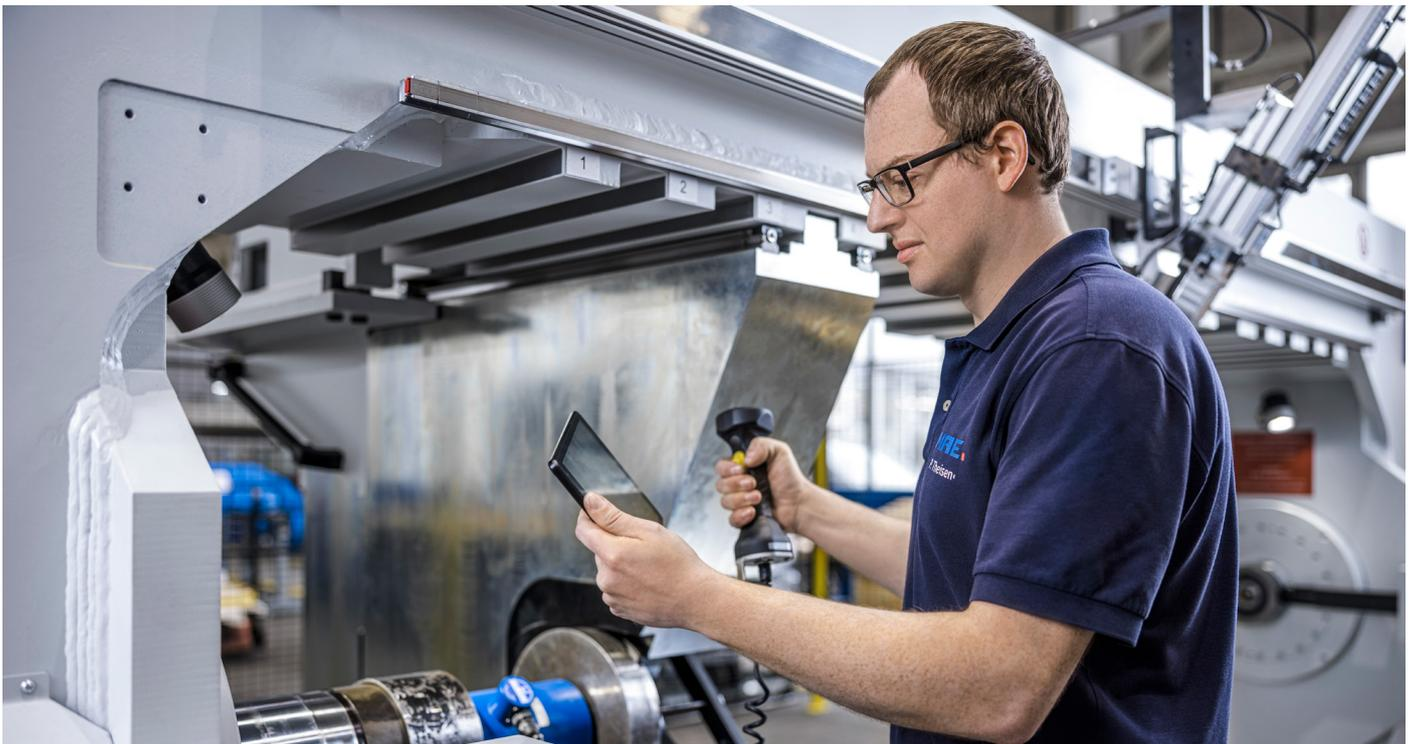
MAE technician during calibration of a wheelset press
