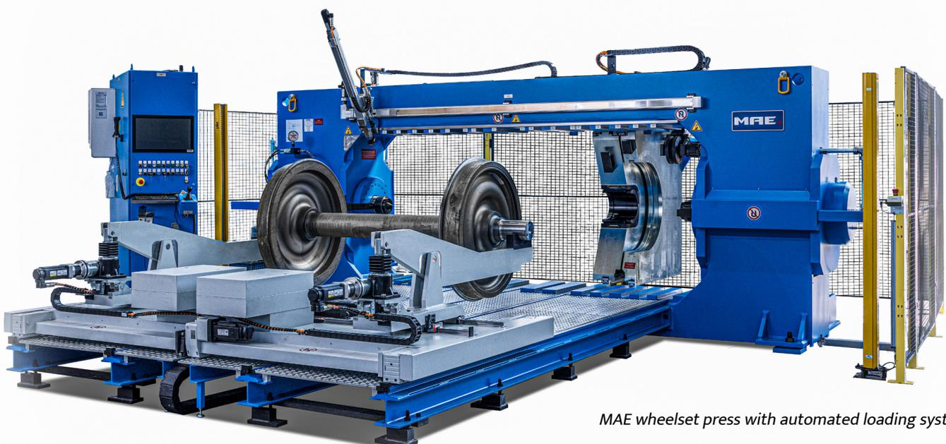
MAE wheelset press with automated loading system
