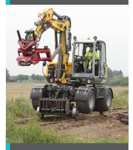
This Hy-Rail attachment is manufactured for excavators 10-20 tons.
