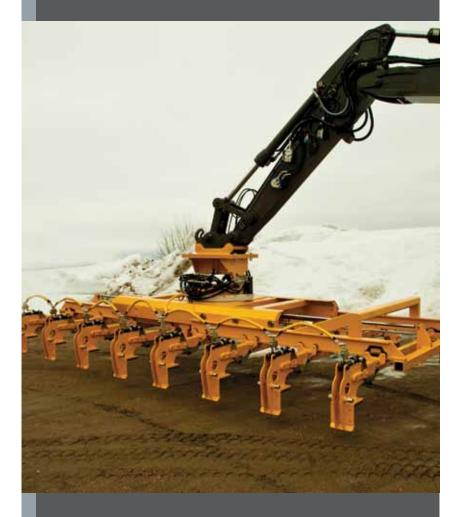
The Sleeper Layer SL850 is designed and manufactured for efficient positioning of concrete sleepers. It utilise standard couplings on heavy excavators and loaders.
