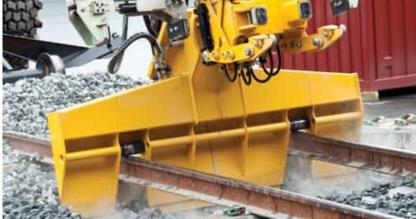
The SB60 Sleeper Replacer is designed to provide safe and efficient replacement of sleepers. It has tilt and rotate functions that allow sleepers to be changed from both the middle and side of the track.
