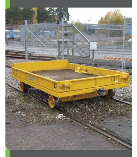
The Rail Trailer RT3235 is designed for transport of material and equipment between different work sites on railway.
