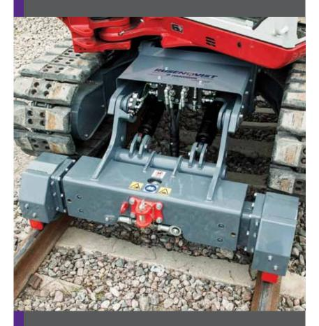
The EQ Axle is designed to protect operators of rail road vehicles RRVs.
