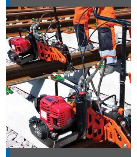
The Handy Clipper is a versatile machine designed for smaller clipping and unclipping applications for the PANDROL FASTCLIP. It has its own power supply and its ergonomic design enhances operator comfort, together with efficient operation.
