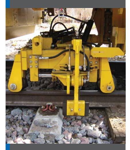
The TRC is an automatic clipping unit for track renewal trains or equivalent. The TRC has an automated PLC-system for fully automated fastening. Built in sensors intents the clips and the clipping tools are fitted to a rigid frame structure and have a hydraulic controlled slide that enables clipping in motion.
