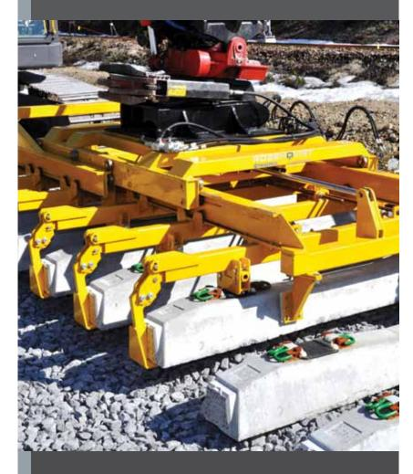
Designed for high output sleeper laying.
