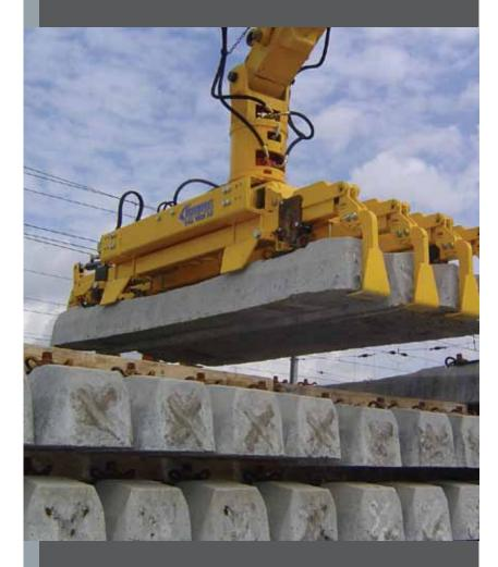
Designed for high output sleeper laying.
