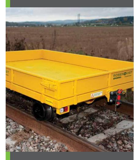
The Rail Trailer RT3230 is designed for transport of material and equipment between different work sites on railway.
