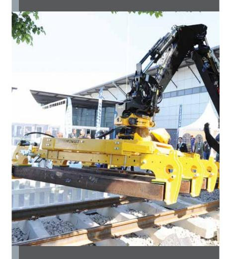
Designed for high output sleeper laying.
