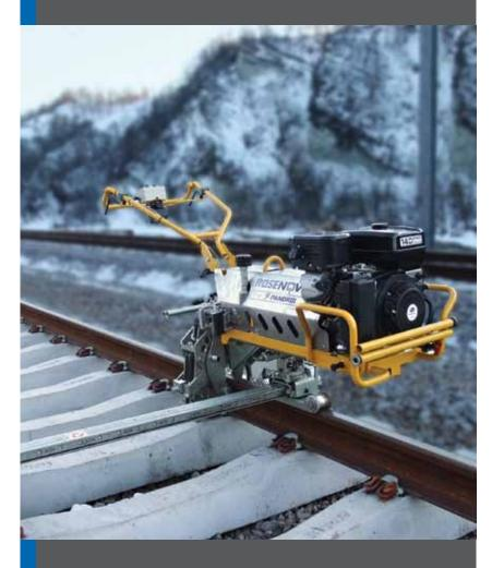
The CD200 is for use by a single operator. It is a high-performance robust walk-behind clipping machine.
