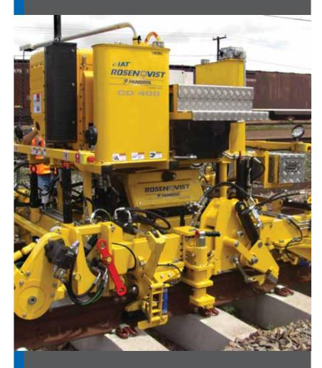
The Clip Driver CD400SP is a walk-behind machine when clipping and declipping clips of the following types: PANDROL FASTCLIP, PANDROL e-CLIPs, PANDROL PR-clips (PR400 series) and Heyback (clipping), depending on the choice of tool. The power pack can be removed when the CD400 is to be used as a conventional machine with a carrier.
