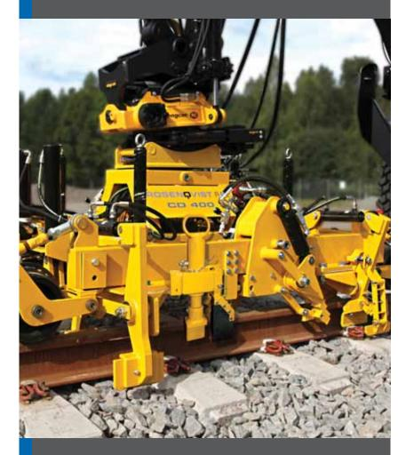
The CD400 Clip Driver is an attachment designed and manufactured for use on a road rail vehicle (RRV) using the host machine's hydraulic power for operation.
