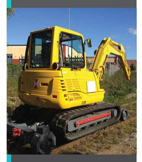
For the most common types of mini excavators. Designed for stability and flexibility. All maneuvering from the driver's cabin. The hydraulics doesn't need extra swivel implements.
