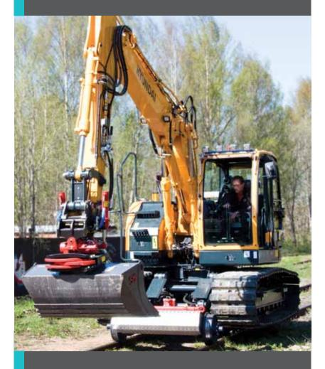
This Hy-Rail attachment is manufactured for excavators 9-14 tons.
