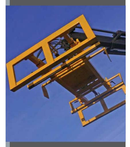
The Sleeper Lifting Tool - SLT 400 is designed to load and unload sleepers from railcars safely and efficiently.
