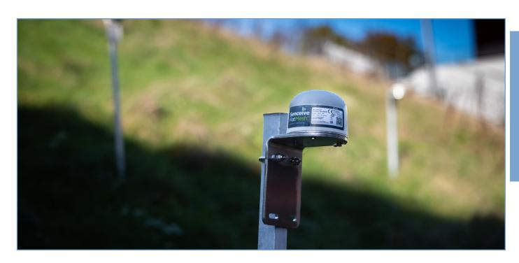
powered, so the system can operate without fixed power or comms infrastructure. Remote users benefit from online datasets typically updated within minutes, along with automated alerts if pre-set thresholds are breached, with increased data granularity based upon the severity of the breach.
