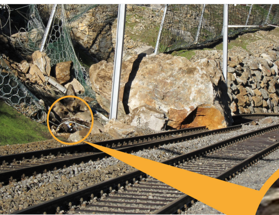
The ImpactSentinel sensor detected a falling boulder breach, averting potential collisions with SBB trains in Switzerland, as seen in the pictures above and to the right, demonstrating its crucial role in railway safety
