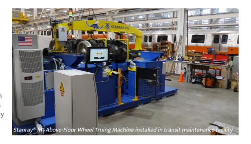
Stanray product line with the new M-Series Wheel Truing Machines. While still employing the same milling machining technology, the new machines include innovations that were not possible when the Stanray was introduced in 1949.
