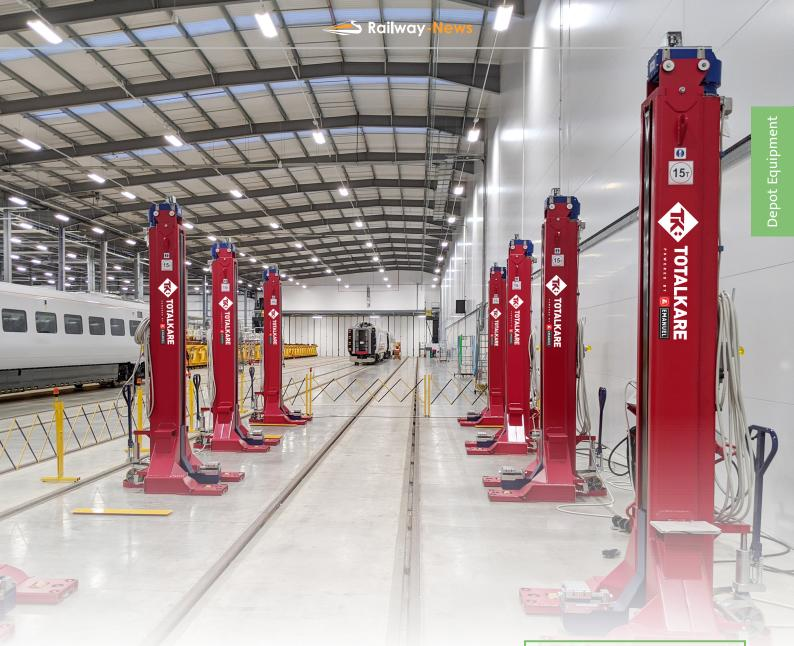
jacks can be configured in sets of four to 128 (facilitating the lifting of a single carriage or an entire train) and are designed to meet Machine Directive 2006/42/CE and approved to European standard EN1493.
