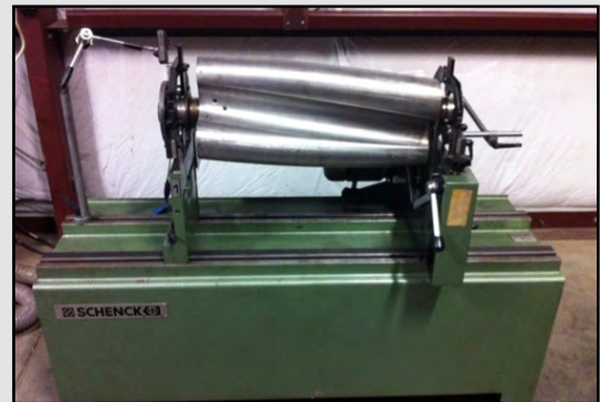
All Scrolls Are Precision Balanced
