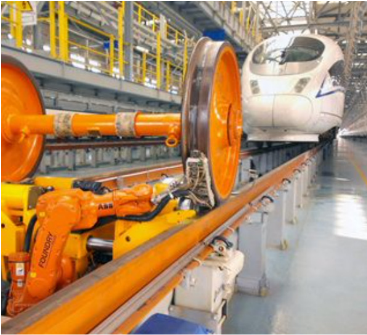
UW-UT system on a calibration reference wheelset (left) and an on-vehicle wheelset inspection (right)
