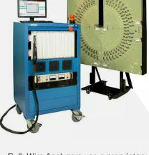
Bulk Wire Analyzers use a proprietary high voltage switching architecture to evaluate and test reels of bundled twisted-pair cable up to 30,000 feet in length for conductor resistance, insulation resistance, conductor to conductor dielectric strength up to 10 kVDC and core to sheath dielectric strength up to 15 kVDC. AC High Voltage testing is available (as a standard offering) up to 6000VAC for 30,000 foot cables.
