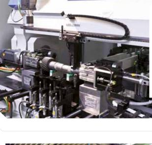
**M.AH 40 straightening system** for gear shafts. Max. straightening power 400 kN, precision up to 0.01 mm run-out.
