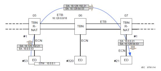
Figure 4 – An example of cross train-car communications
