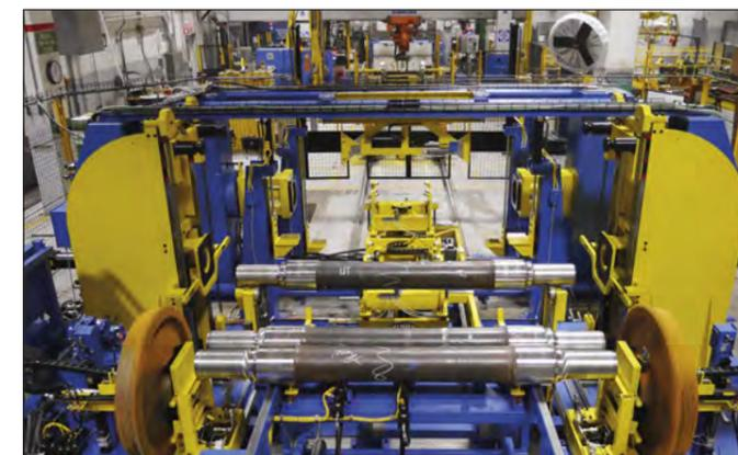
Automated Wheel and Bearing Mount Cells
