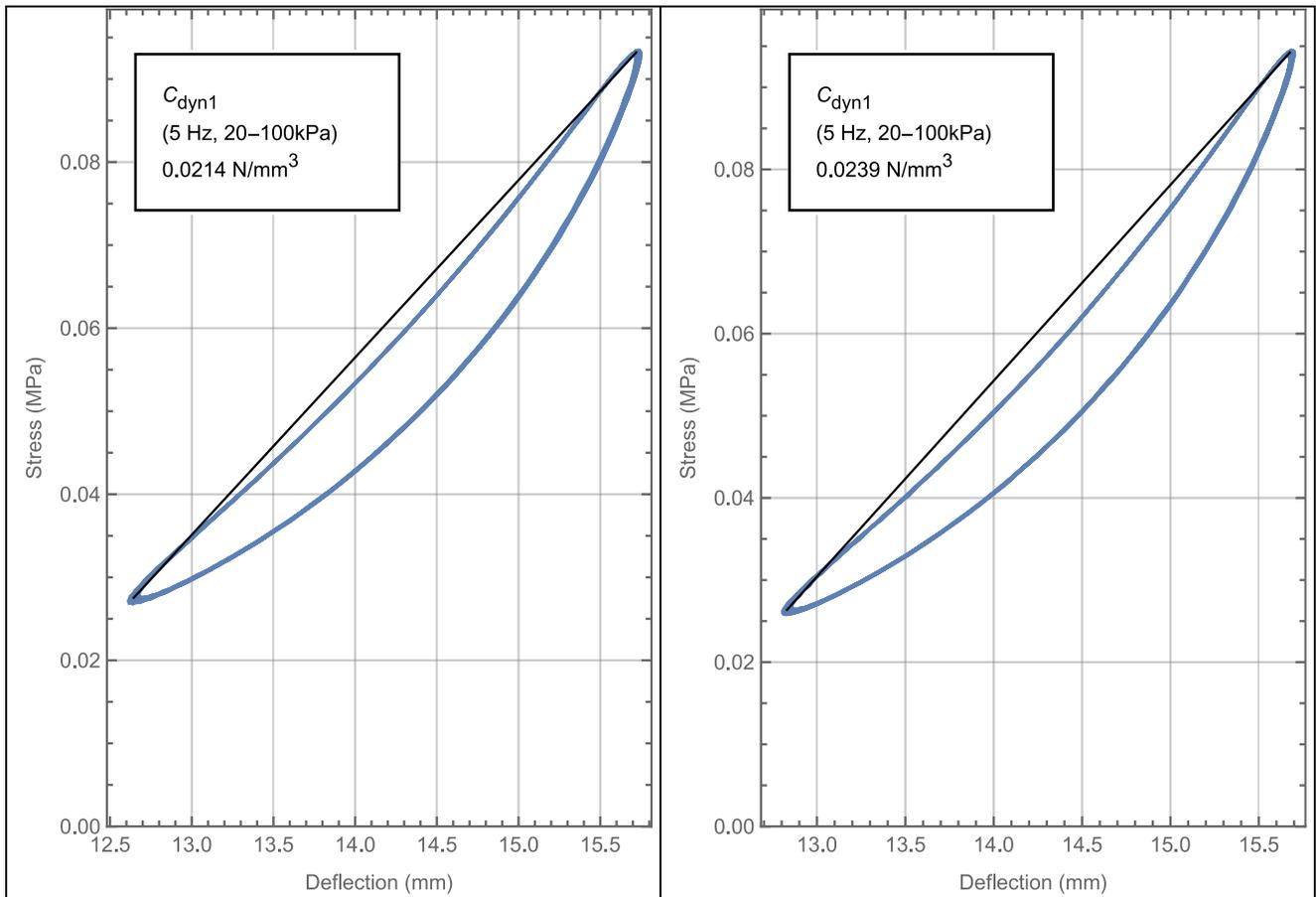
Figure 5: Example of  $C_{dyn}$  (5 Hz, 20-100 kPa) measured before (left) and after (right) 3M cyclic loading.
