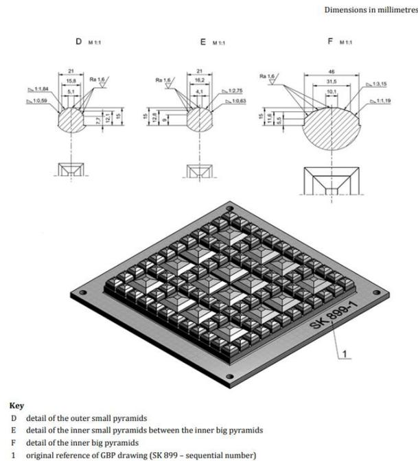
Figure A.2 — Details and isometric view of GBP
