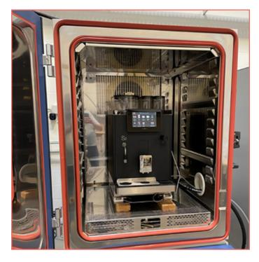
In the Damp Heat, Cyclical test, conducted according to EN 60068-2-30, the S2 Railway was exposed to extreme humidity levels (90–100% relative humidity). This ensured its durability and performance under harsh conditions.
