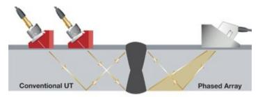
Phased array testing compared to conventional UT. The ability to test welds with multiple angles and depths from a single probe can increase the probability of detecting an anomaly.
