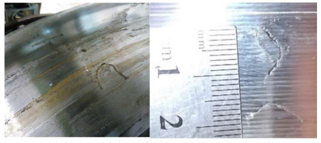
Wheel fatigue crack findings (left) before and (right) after tread reprofiled
