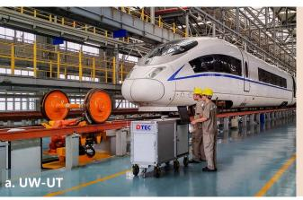
Our Underfloor Wheelset Ultrasonic Testing System (UW-UT) is designed to perform highly efficient, accurate, and highly reliable wheelset inspections under the train. With our Underfloor Vehicle Bogie Machine Vision System (UVB-MV) using Artificial Intelligence, 3D imaging, and robotic automation techniques, we are moving the asset management into a new era of smart maintenance.
