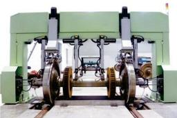
Dismounted wheelset and solid axle ultrasonic testing systems
