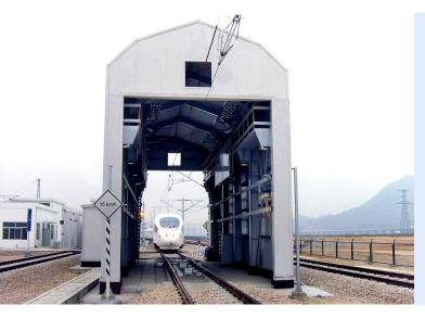
Check Point / Tunnel, installed at the trackside, consists of many modular function units, and is designed to carry out various inspections and measurements for a moving train. This includes monitoring of the wheel profile, detection of wheel cracks by ultrasound, measuring of brake pad and pantograph carbon strip, as well as fault recognition for other visible key components, such as lost bolts, adhering foreign objects by machine vision.
