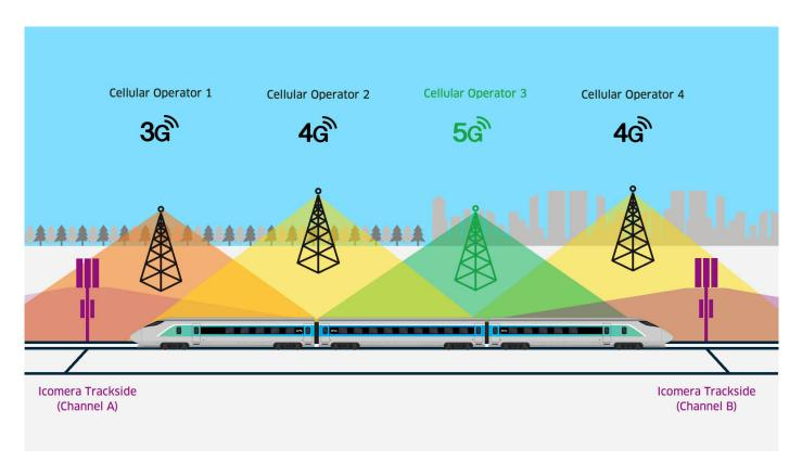
Icomera's SureWAN technology aggregates multiple communications networks, providing the fastest, most reliable Internet connection available to a moving vehicle
