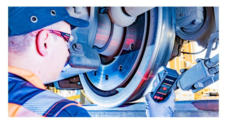
With its unique CALIPRI® technology from NEXTSENSE, Hexagon is one of the world leaders in mobile profile measurement systems for wear measurement of wheels, rails and tracks.
