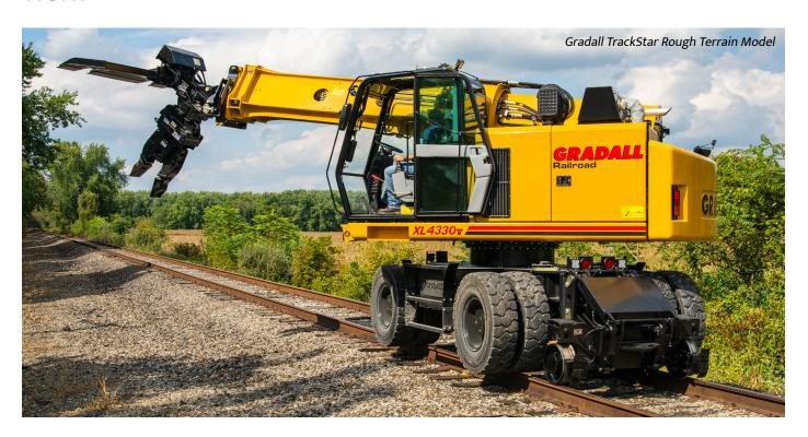
Gradall railway maintenance machines represent a unique combination of mobility and versatility, able to get to the job – either on rails or pavement – and then efficiently handle a wide range of maintenance and construction jobs.
