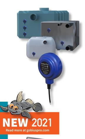
You could say "Knock and listen" but it's more sophisticated than that. A Gobius sensor exerts force onto a tank wall and causes it to vibrate. An accelerometer is part of the sensor and it measures the vibrations. The processor's algorithm calculates a vibration value each time the sensor performs a measurement.
