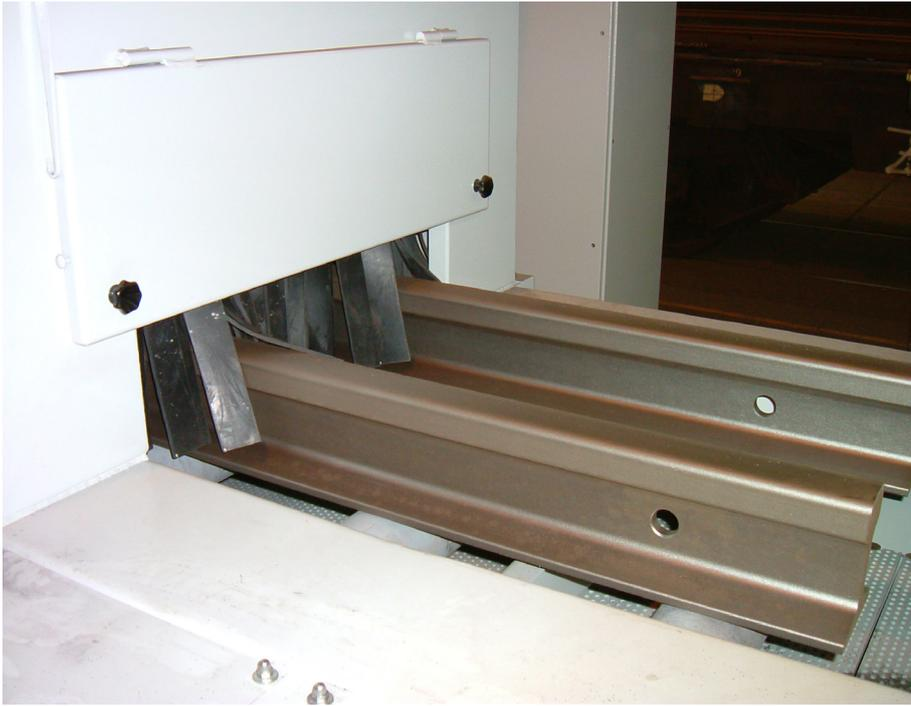
to fatigue failure too. Shot peening increases their fatigue strength and lifespan, raises the maximum working load and prevents sagging.
