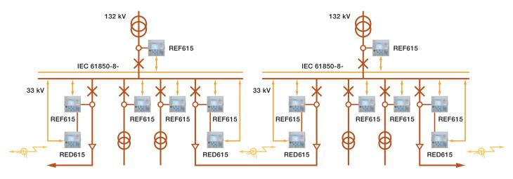
IEC 61850 provides protection and control for rail applications
