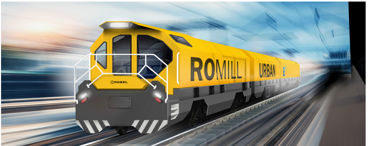
ROMILL Urban E 3 has been designed for emission-free rail treatment in subways © Robel
