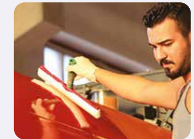
Step 12: Applying the permanent coating - Permaseal TP.
