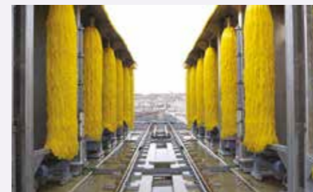
Permanent carriage wash machine
