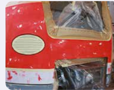
Step 7: Masking off the areas to be painted.
