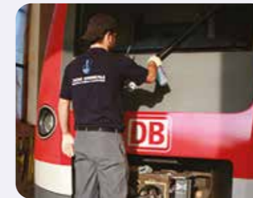
Step 11: Preparing the old surfaces for the permanent coating.
