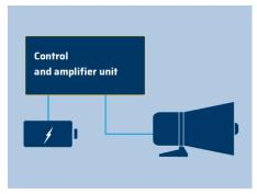
The electric actuation of our electrical Makrofons offers a signalling variant that is quickly operational and is independent of the compressed air supply
