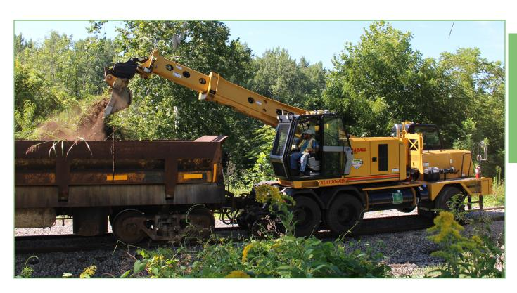
like replacement ties or riprap, means one operator and one machine can accomplish more, streamlining logistics and labour.
