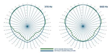
The sound pressure level decreases towards the rear/towards the driver's cab when the sound insulation is installed
