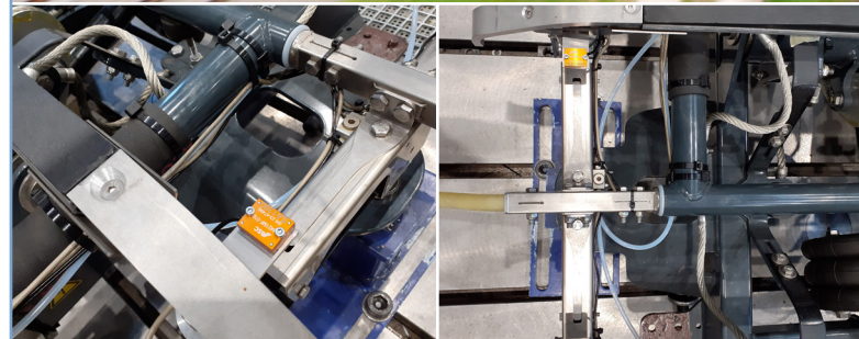
ASC 4421MF accelerometer used in pantograph testing at 350+ km/h © ASC Sensors
