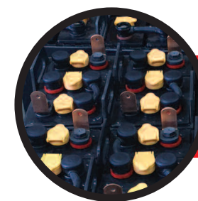
MK3 Coach Wet Lead Acid Auxilliary Battery
