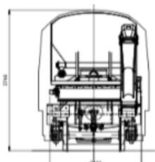
**BODY:** Continous mixing equipment with separate storage for materials
