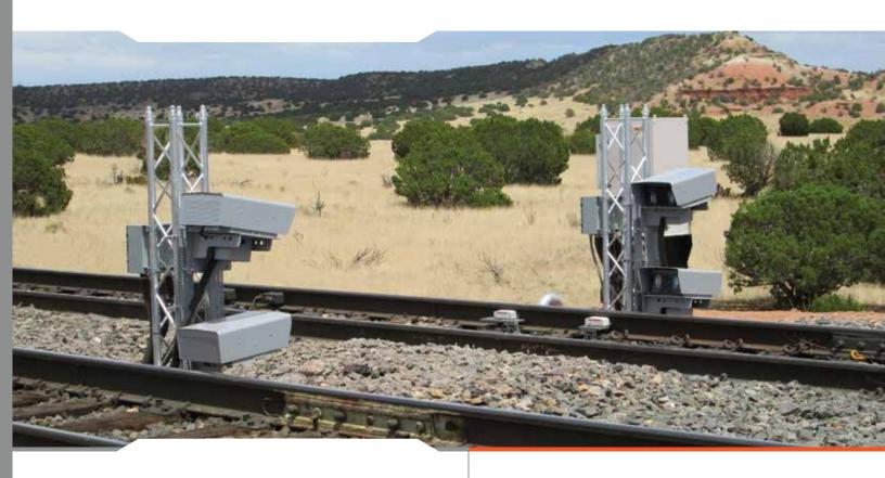
BrakeView-Shoe is a wayside brake shoe (Block) Measurement system designed to inspect brake shoes at track speeds. This system is vision-based and uses a multi-camera high speed imaging unit to take multiple images of every brake shoe for inspection and measurement.
