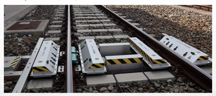
To enhance their rail vehicle maintenance operations, Wiener Linien selected Hexagon's CALIPRI X automated wheelset measurement system because of its quick, exact and reliable wheel profile measurement capabilities.
