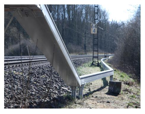
Size 2+ has deeper and more robust side walls, designed to withstand higher lateral loads than Size 2, enabling the system to withstand the pressure from snow ploughs clearing snow drifts. The deeper design also allows for multiple cable jointing where necessary.
