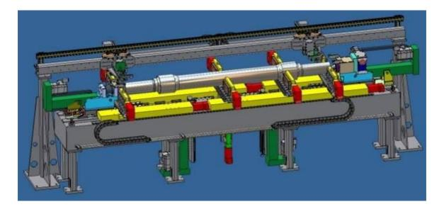
Using a crane, a worker loads the axle into loading prisms, which safely slide into the measuring position. The axle is rotated by two centring pins, one of which is powered by the servodrive.
