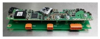
Figure [3] – Amantys Gate Drive Adapted for legacy traction converter
