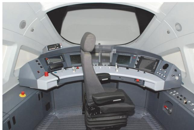
In order to ensure fidelity and to provide a very realistic training environment in form, function and feel, the control desk will replicate the control desk of the real train, incorporating all the indicators & gauges, control levers, switches, flashing and audio warnings, visual and functional aspects as true to the real cabin.
