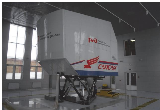
Replica cab and display system will be mounted on top of the motion system, providing the driver with the highest level of immersion into the simulated / virtual railway operating environment.
