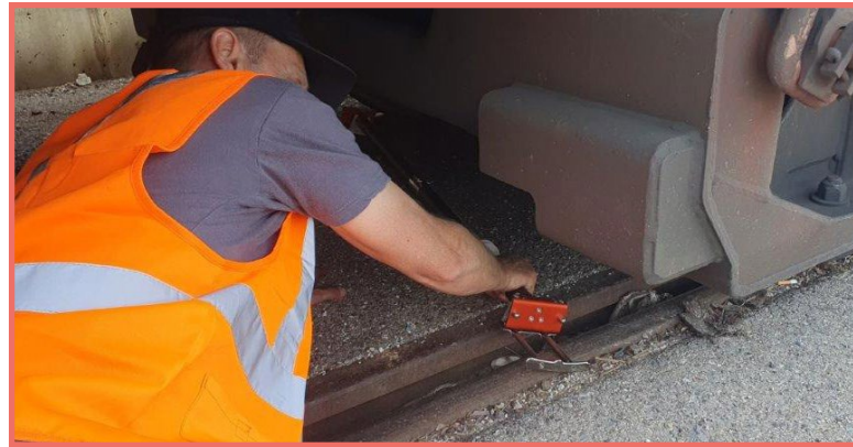
An employee from the team measuring the inner clearance within wheelsets, this measurement is a challenge for wheelsets of freight vehicles
