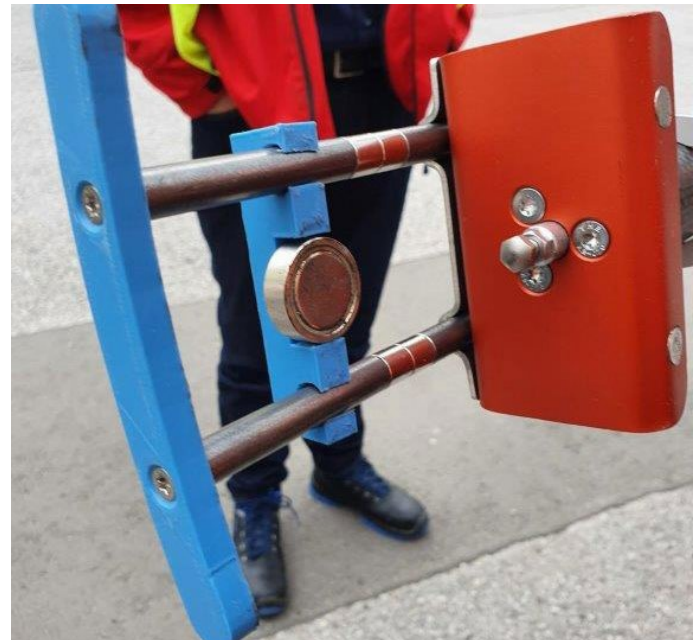
The gauge has more robust contact surfaces and an adjustable length, making it easier to handle
