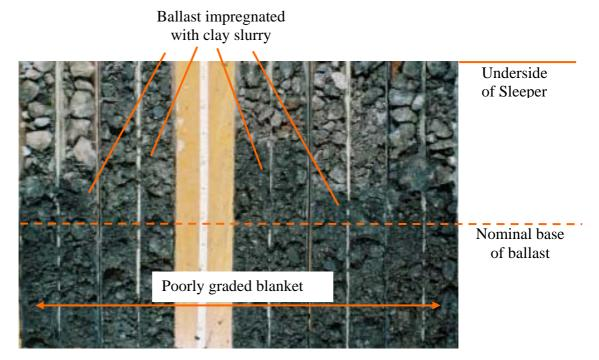
Figure 2 Boreholes taken through trackbed with poor quality blanket.
