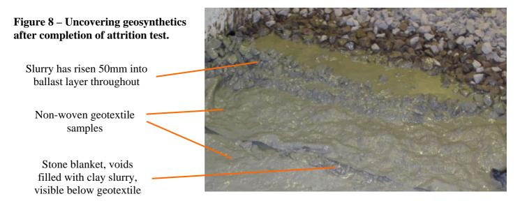
Assessment was made by measuring the area of the holes in each geotextile. A piece of graph paper, area 124,800mm<sup>2</sup> was placed under each geotextiles in the worst area of damage, which appeared to be in the position beneath the end of a sleeper. Holes were marked by tracing with a soft leaded pencil onto the paper behind. Measurements were made of the area bonded by each pencil mark in turn and the total area calculated in each case. Table 3 gives the results of the tests.
