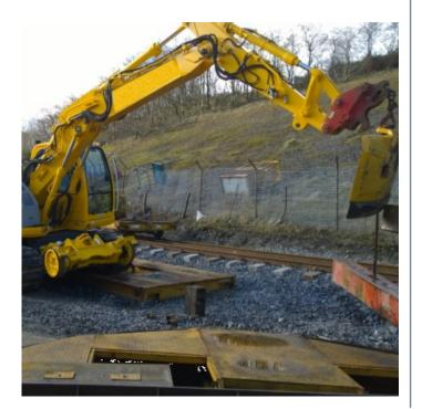
SpaceGuard increases productivity by enabling the machine to be able to operate at all times even under live overhead wires (OLE) or next to open traffic lines (ALO). SpaceGuard is currently the only electronic safety system in use on the rail complying with UK requirements for live overhead wires and open traffic lines.
